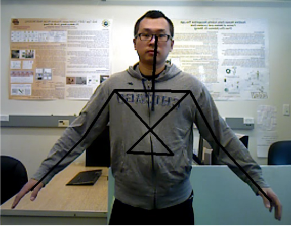
Fig. 6. Human skeleton tracking by the RGB-D sensor.
