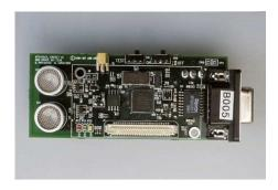
Fig. 2. The Cricket sensor node.
