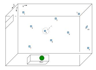
Fig. 3. Schematic representation of lab layout, from above. Sensors 1-4 and 6-9 are affixed to the ceiling (z=0). Sensor 5 hangs from an overhead light, 95 cm below the ceiling, and sensor 10 is attached to a wall at z=128 cm.
